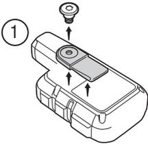
1 Remove the webbing loop with a hex wrench included with the Garmin Mini.
