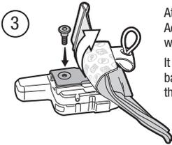
3 Attach the Garmin Mini Spine Mount Adapter with the LONG bolt included with your device. It is helpful to fold the Tracker Packer back during this process to expose the bolt hole.
