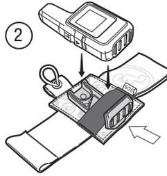
2 Slide the Garmin Mini Spine Mount Adapter under the webbing strap.
