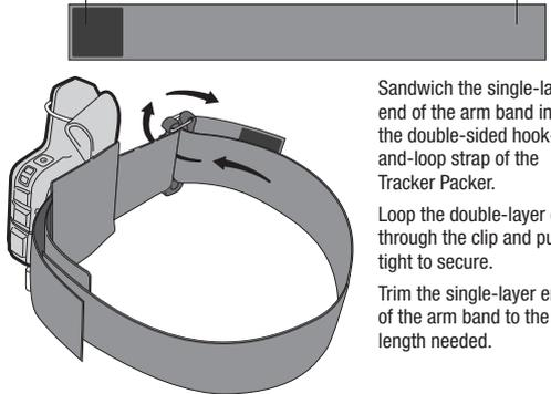
Sandwich the single-layer end of the arm band into the double-sided hook-and-loop strap of the Tracker Packer.
