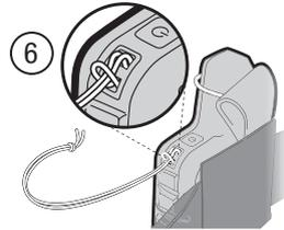
6 Girth hitch the tether to the Garmin Mini and use it to attach the device to your backpack or apparel.
