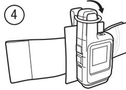
4 Fit the elastic loop over the antenna.
