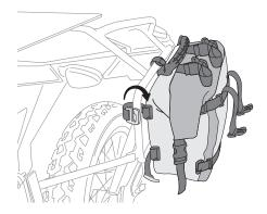
**IMPORTANT! INSERT ALUMINUM HOOK INSIDE THE** WEBBING LOOP, NOT AROUND IT.
