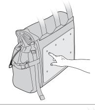
Use a ball point pen to mark hole locations where the mounting hardware passes through the Pannier. Repeat on second Pannier.
