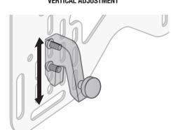
Use one of the four slot positions to locate mount hooks where they clear obstructions and hot exhaust. Adjust hooks vertically in slots for a tight fit when the quick-connect clasp is attached to the rack
