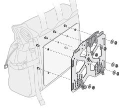
**INSTALL ONTO LUGGAGE RACK** Once GL Pannier Mounts are installed on RTW Panniers, hold by the handle and drop hooks onto luggage rack, pulling quick-connect clasp open and allowing it to click into place. Lock Panniers to luggage rack for maximium security and to prevent accidental
