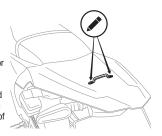
Drill holes through the fender in marked locations.
