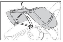
Position saddlebag as desired, secure hooks on either side of fender.
