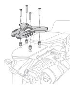
Insert each of the four spacers inside the rack mount holes. Lay the rack over the spacers, careful to align the holes with the spacers underneath.
