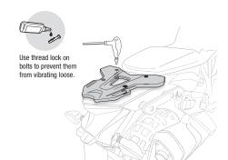
Finger tighten all four bolts into place for several turns to avoid cross threading. Use the KTM tool to tighten.
