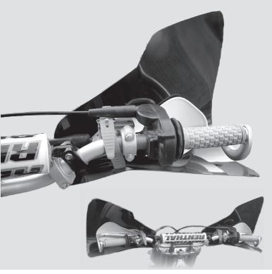
Motorcycle must be equipped with rigid handguards or deflectors to support Bushwackers while riding. Failure to follow recommended mounting and installation instructions voids warranty. Manufacturer is not liable for any damage, injury or death that results from improper use and installation of products. By installing these products, user accepts all liabilities, terms and conditions outlined in the Liability & Warranty statement included here.
